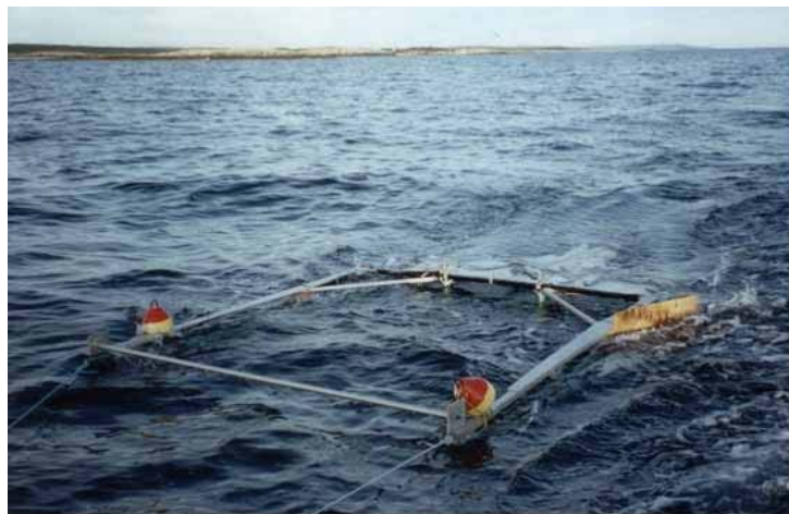
Figure 2. View of plankton net and frame towed behind a fishing vessel. Note the wooden deflector on the right-hand side of the picture.
