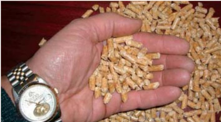
*Premium Pellet Ltd. makes wood pellets by drying the raw material, pulverizing it and then compressing it into small pellets that are smooth to the touch.*
